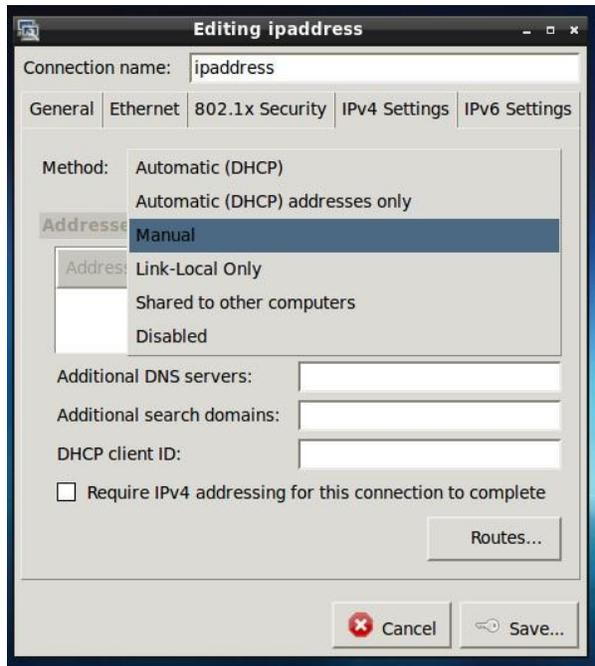
Now the desired static ip parameters can be given by clicking the “Add” button and entering the parameters as shown below.
