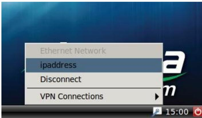
To view the current IP address of the system, user can “Right click” the “Network Settings” item on the taskbar and click on “Connection Information” as shown below.
